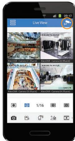
**7** Double tap a channel to view it full screen. Pressing the camera list icon allows you to choose which cameras are displayed.
